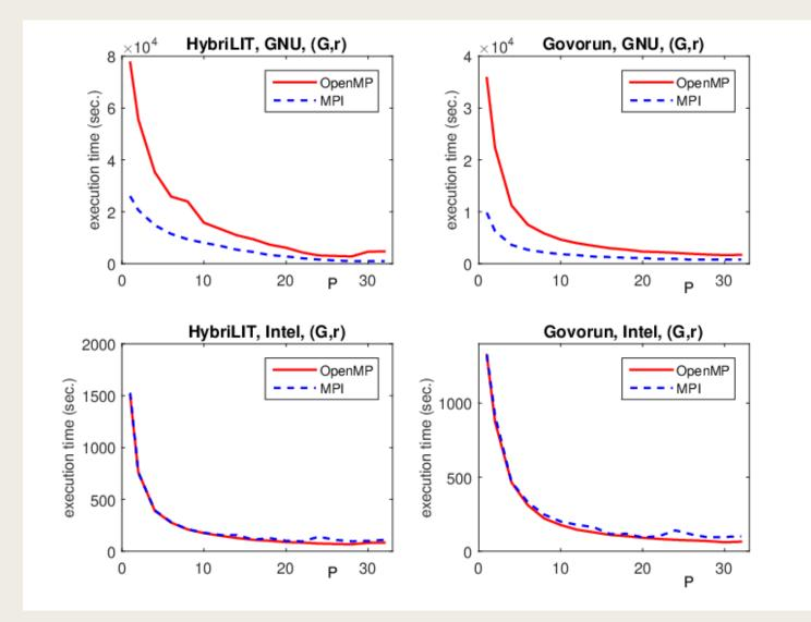
Time of calculations depending on the number of MPI-processes/ OpenMP threads.
